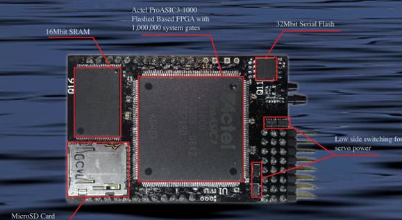
At only 40x60mm in size, Asity has been designed to fit into the cramped narrow fuselage of efficient, scale gliders, while still containing all components required to operate and communicate with an autonomous UAV.
